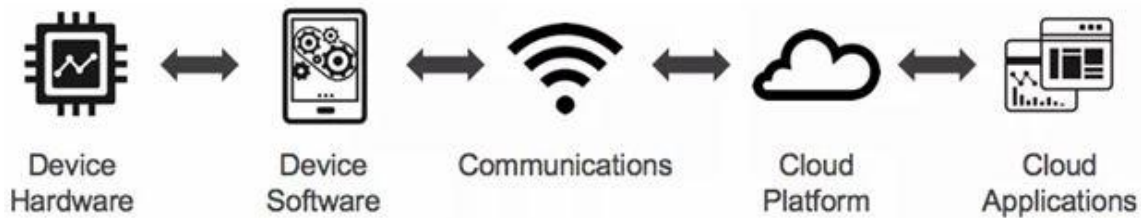
Figure 3: The IoT Technology Stack.
