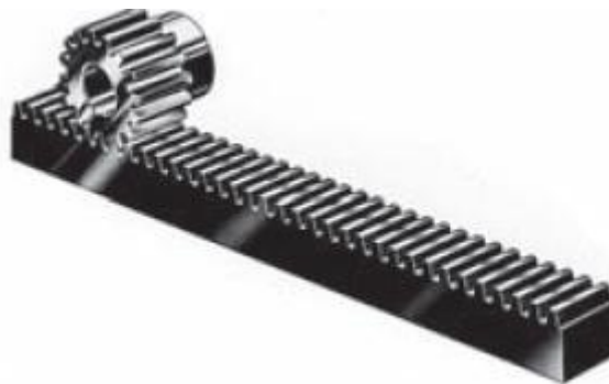
Figure 1. Representing the Rack and pinion gear research gate [Made in China].
