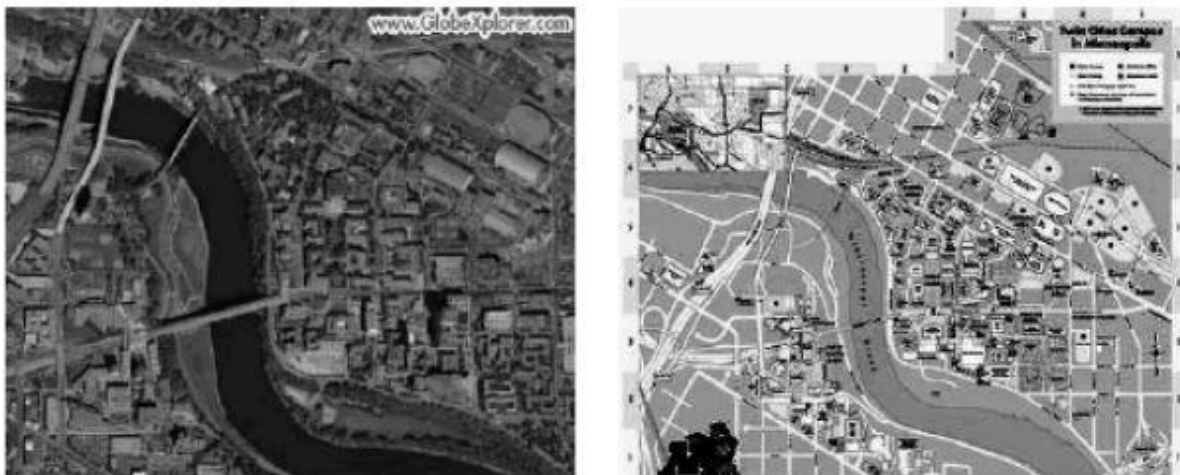
Figure 1: The above figure shows the raster and vector data for a campus.
