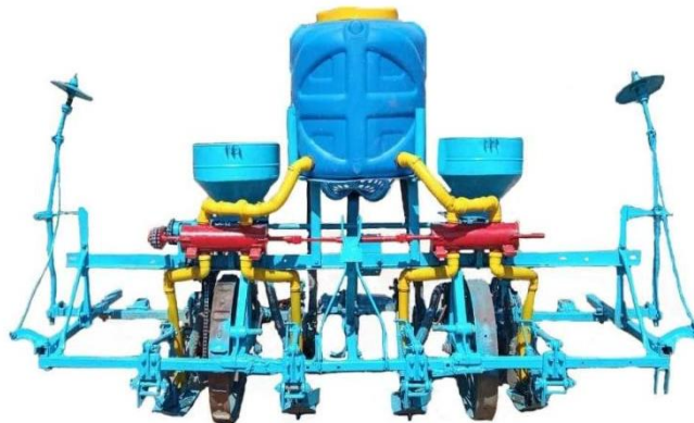
Picture. 1. Seed planting device with improved liquid organic fertilizer.
