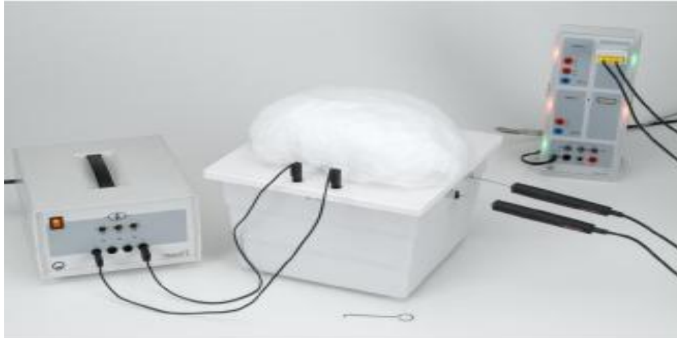
Figure 2. A device for determining the thermal conductivity of a sample of a building material using the single plate method
