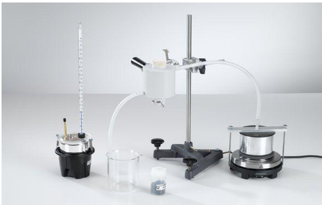
Picture 1. Determination of specific heat capacity of solids experimental device for. 2-
