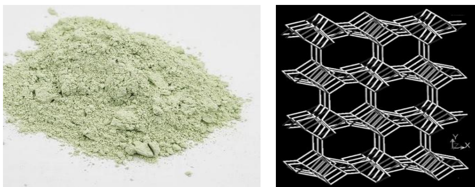
Figure 1. Projections of montmorillonite and montmorillonite structure.
