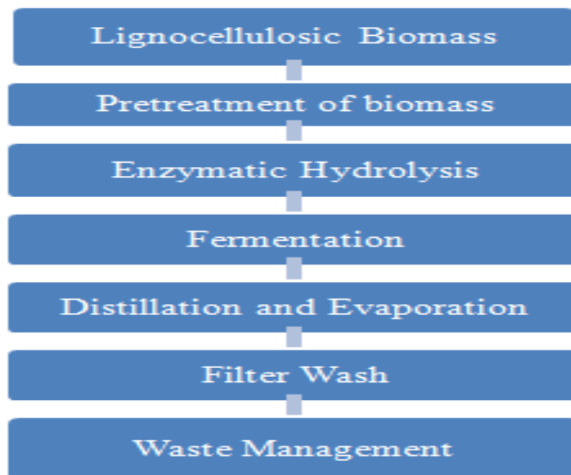
Figure 1: Illustrates the overview of bio-ethanol production process
