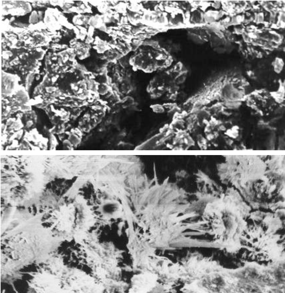
Picture. From processing of concrete structure with Mobet material previous (a) and subsequent (b) electronic images
