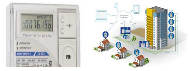
Tasks of the ASKUE as a measuring system. The main purpose of electric energy accounting is to obtain reliable information about the amount of produced, transmitted, distributed and consumed electric energy and capacity in the wholesale and retail market.
