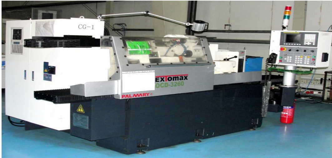
Figure 2: Cylindrical Grinding Machine Source: GTDMC Machining EXTOMAX (OCD-3260)
