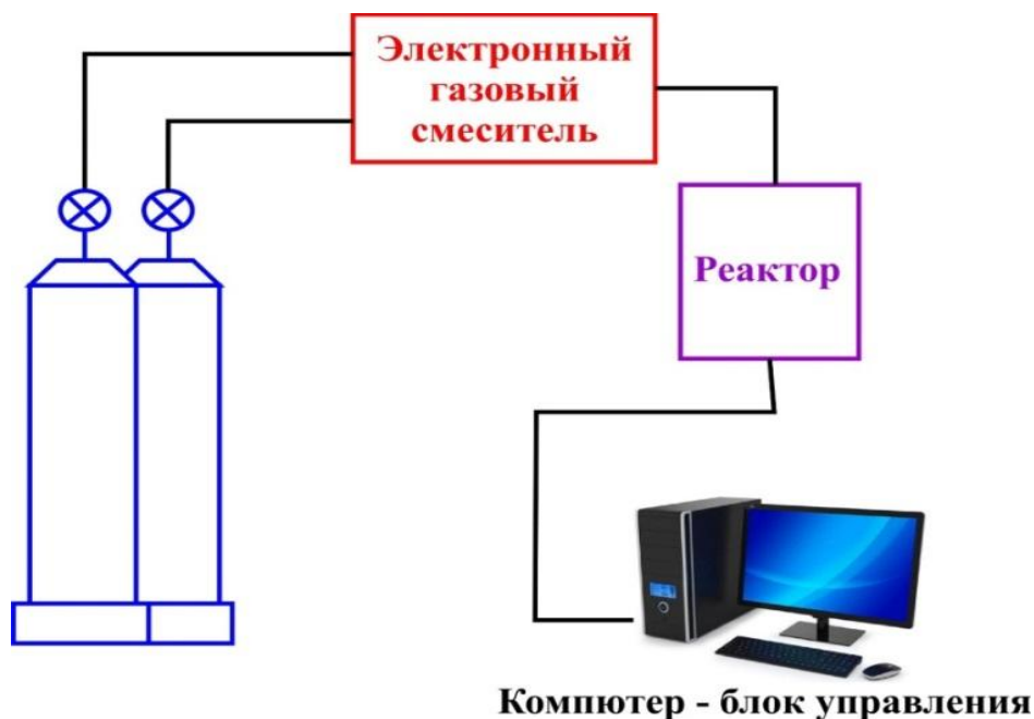
Figure 6. Device scheme for determining the kinetics of the process of formation of carbon nanotubes
