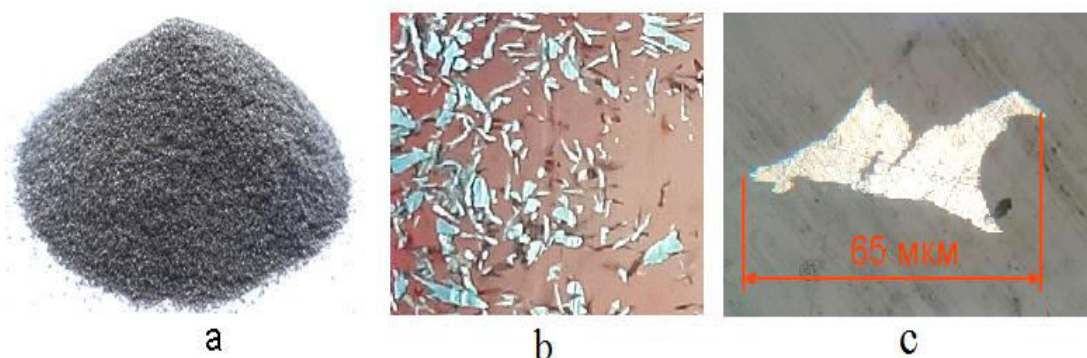
Figure 1. Aluminum powder from ADS-12 brand aluminum scrap: a - general appearance; b - particles (x250); c - particle shape (x650)
