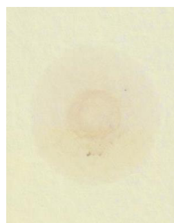
Tellus 463790 moto / hour Hydraulic excavator RH-40E is a working fluid filtered according to method 1
