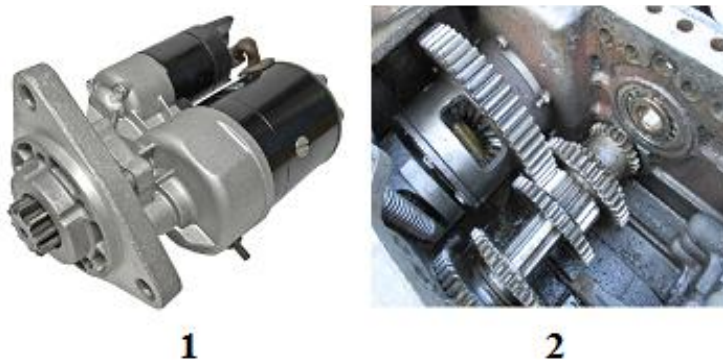
1 2 1-Gear starter; 2-Transmission box
