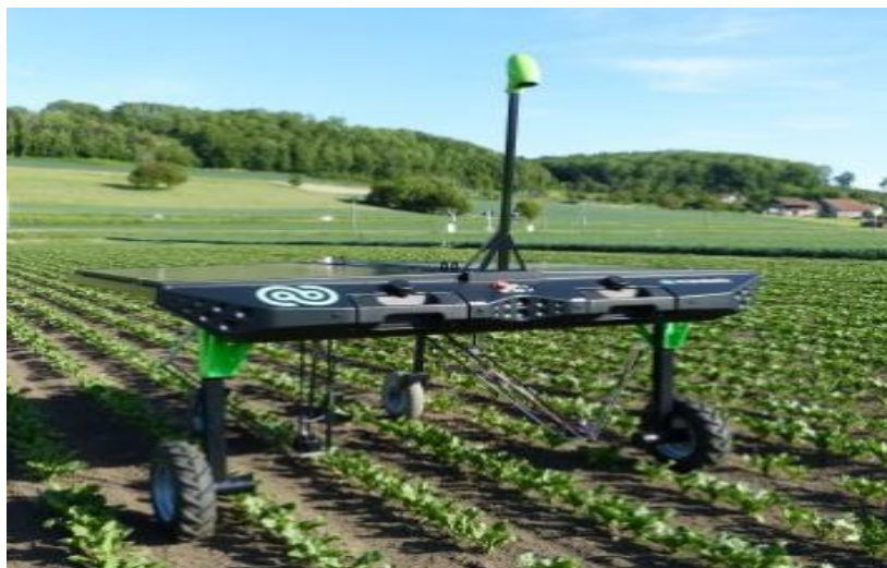
Figure 1: illustrate the Solar-powered robot from ecoRobotix[6].
