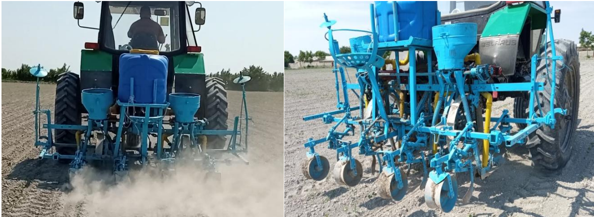
3 Pictures. The working process of the seed drill with liquid organic fertilizer.
