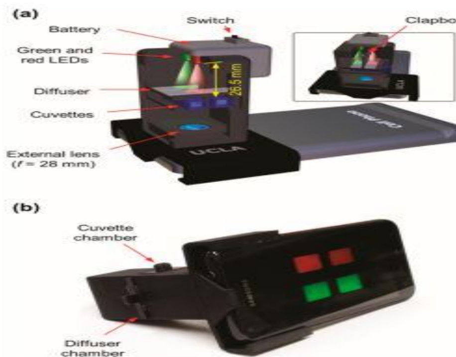
Figure 1: The above figure shows the Design of the ratio metric optical reader on a smart-phone.
