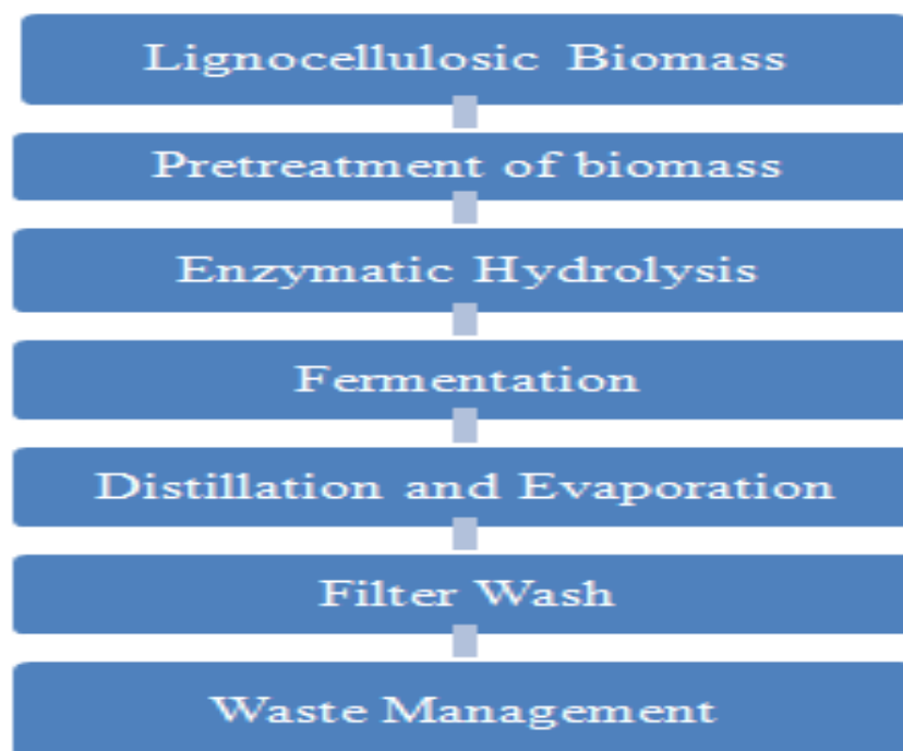
Figure 1: Illustrates the overview of bio-ethanol production process
