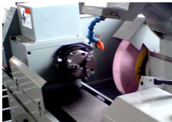
Figure 3: Headstock Position on Cylindrical Grinding Machine. Source: GTDMC Machining EXTOMAX (OCD-3260)
