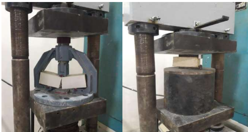
Figure 1. Determination of bending and compressive strength of gypsum; a) bending, b) compression
