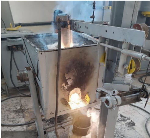
Steel melting process in an electric arc furnace in the laboratory of the Casting Technology Department
