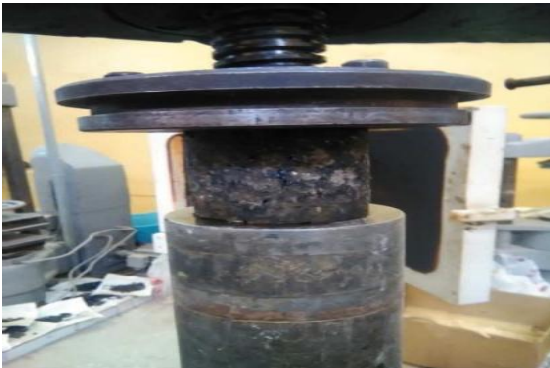
Picture 1. Process of verification of prepared asphalt concrete in hydraulic press.
