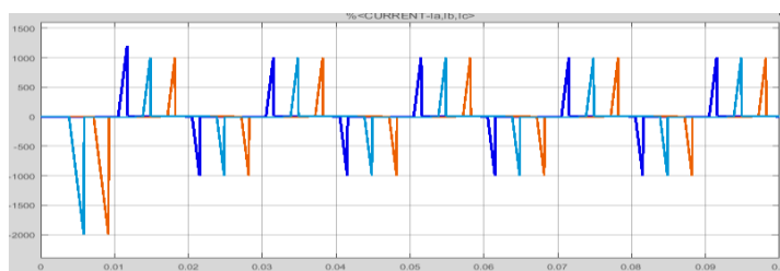
Fig.30. Output phase current waveforms of I_a , I_b , I_c for three stepped three phase inverter
