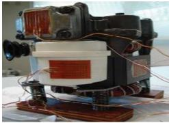
Figure 3: Use of Heat Flux Sensors in Refrigeration Compressors.
