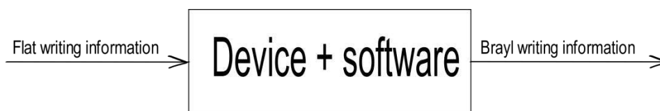
1-picture The principle of a Braille translator
