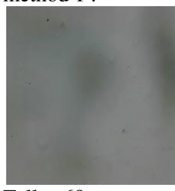
Tellus 68 3088 moto / hour Hydraulic excavator RH-40E Composition of working fluid, filtered according to method 1 .
