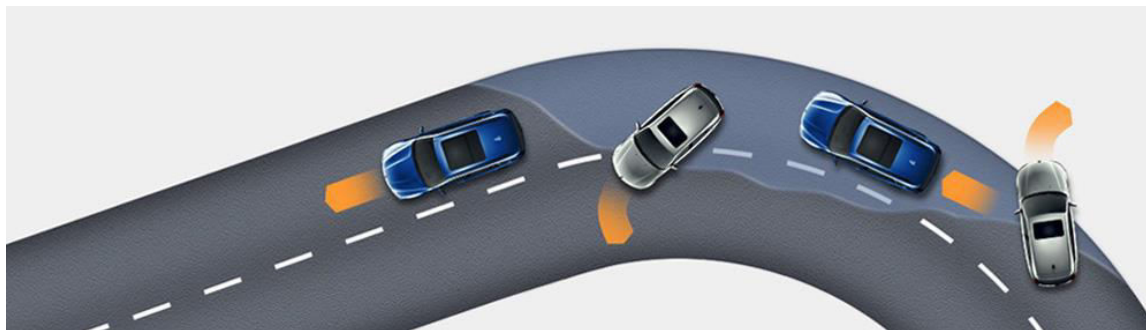
Figure 2. Probable motion of a vehicle with a high-speed ASR system (blue) and a vehicle without (white).
